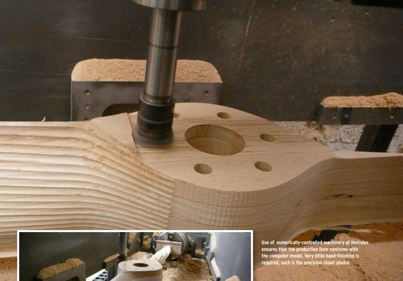
Use of numerically-controlled machinery at Hercules ensures that the production item conforms with the computer model. Very little hand-finishing is required, such is the precision (inset photo)
