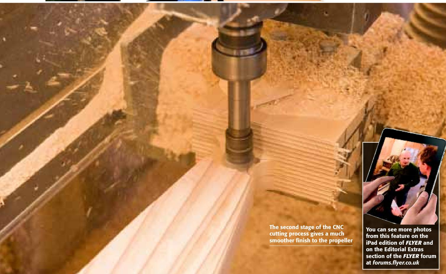
The second stage of the CNC cutting process gives a much smoother finish to the propeller
