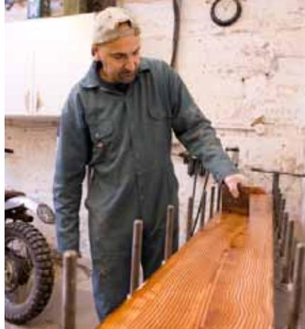
**Left: George applying the Aerodux glue before the beech sections are clamped together.**
