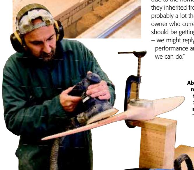
**Above: while the CNC machine makes some early in-roads into the laminated beech, George Simoni (left) skillfully polishes a nearly-finished propeller**
